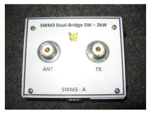
The dual 200W / 2kW measurement bridge
