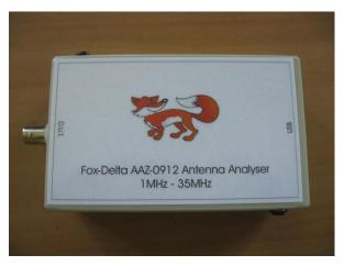
The 1MHz – 35MHz antenna analyser
